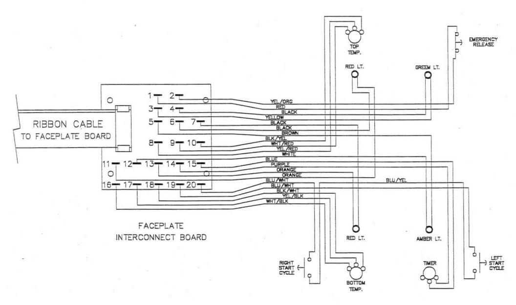
MODEL ES-30 and MODEL ES-32 (with 5"x6" PLATENS) MACHINE BASE SCHEMATIC
